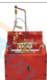
GS-2000PLUS (Precision valve seat boring machine)
